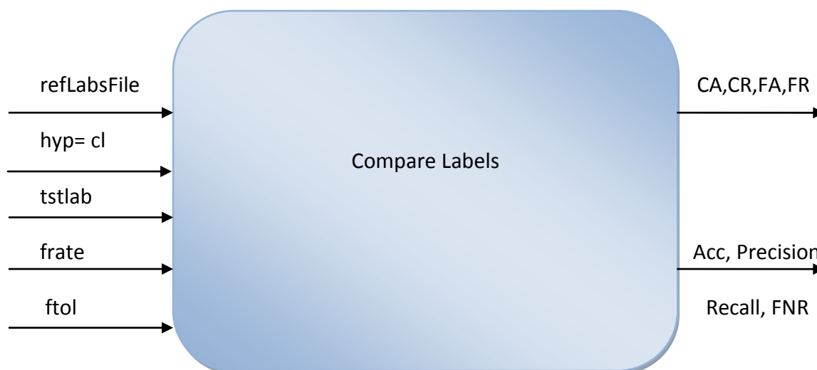
Figura4.6- Block diagram of the evaluator
