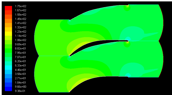
Contours of velocity magnitude. Structured grid
