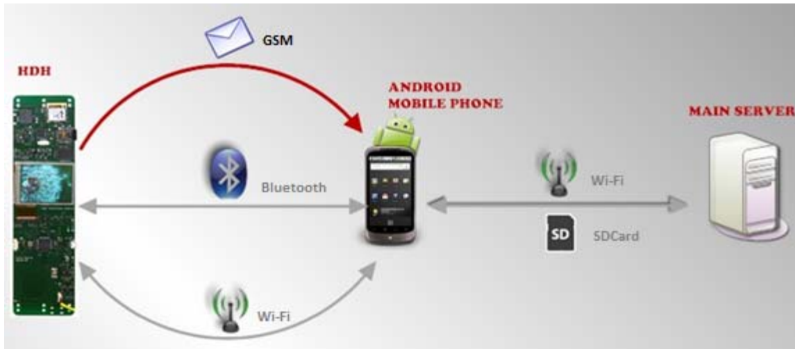
Figure 3.21 GSM connection HDH-Android Server
