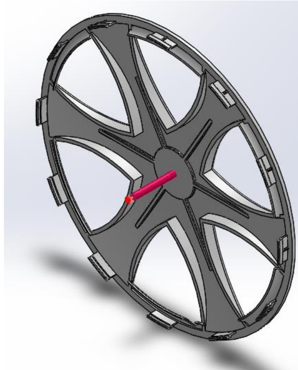
Figure 30 Inlet flow channel and injection point
