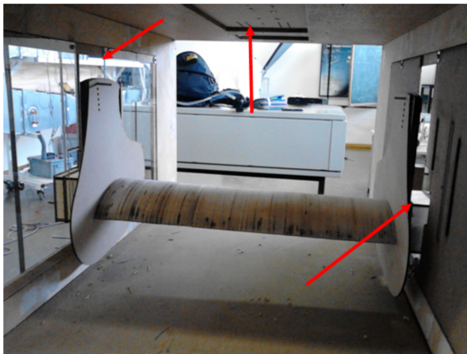
Figure 59 - Gaps and defects of the aerodynamic section
