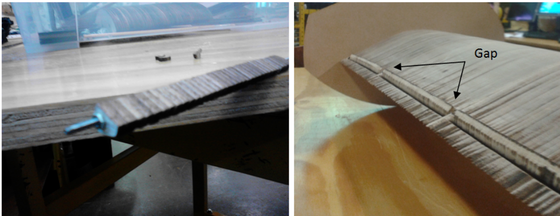
Figure 37 – The microtabs joined in the metal rod (a); gaps in the blade span (b)
