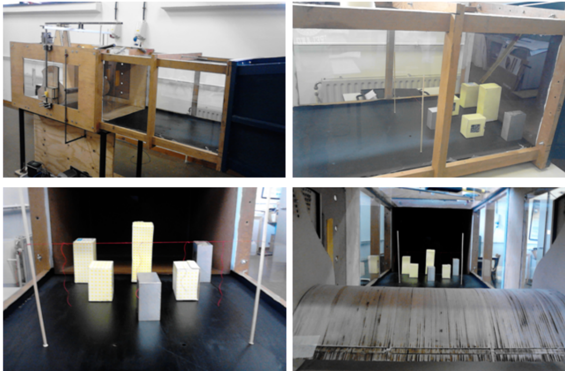
Figure 63 – Set up for the test of increased turbulence
