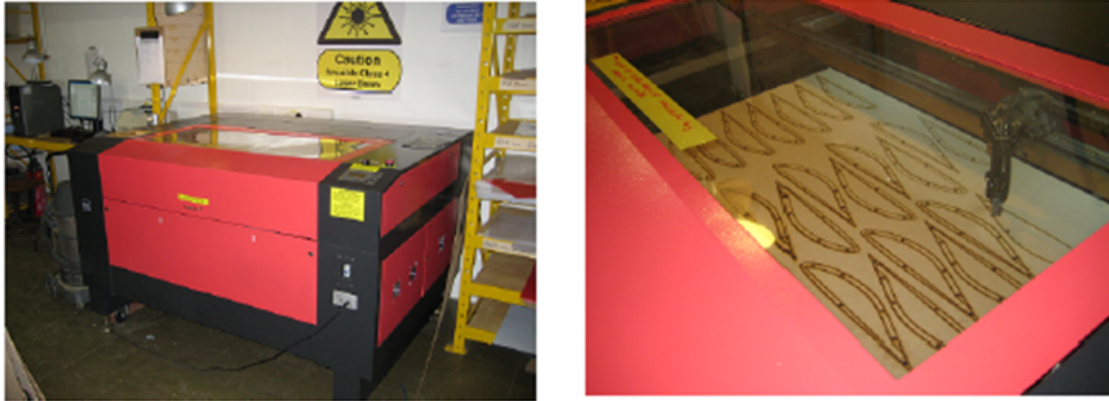
Figure 28 – The laser cutter in the FabLab and cutting wood sections
