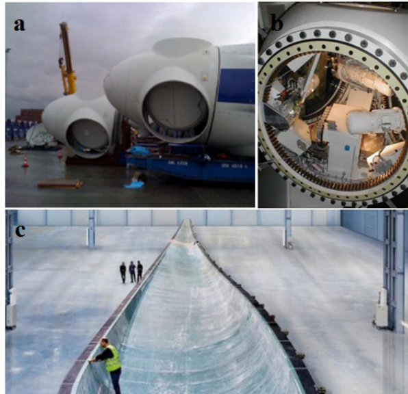
Figure 11 – a) rotor hub; b) rotor hub with actuators and sensors inside; c) mould for the construction of the blades [5]
