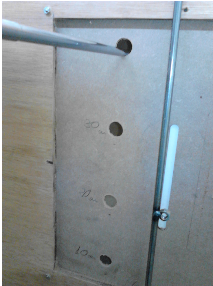
Figure 62 – Holes at different heights (10-20-30-40 cm) located before the blade in the tests section
