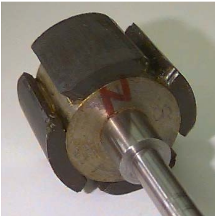
Fig.3.5 Permanent magnet rotor with two pairs of poles[8]
