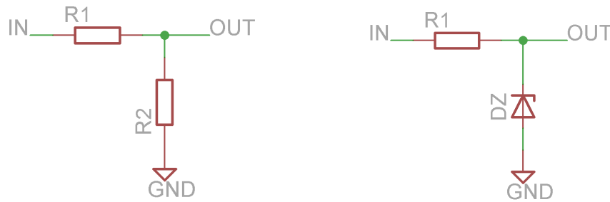
Figure 2.3.: Implementations of the voltage divider with the resistors and the Zener diode.
