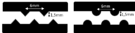
Figure 3.27. Microbender sensors teeth geometry.
