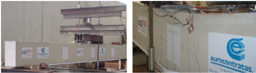
Figure 6.8. Pre and Post bending test beam pictures.
