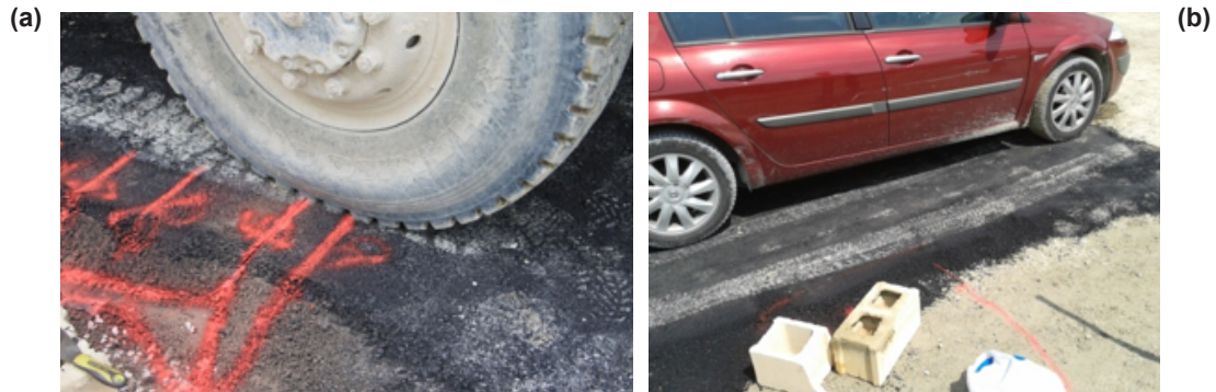
Figure 6.20. Pictures of the sensitivity test when different loads are placed over the sensors.
