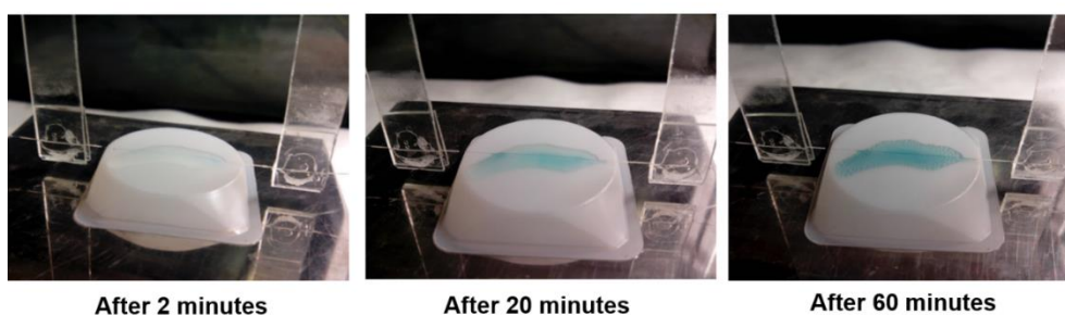
Fig. 4.18. Presence of AGAs in the T-SMF proved by using the TMB - HRP enzyme method [23].
