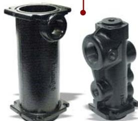
**HEATING & COOLING CYLINDERS...** separate heating and cooling cylinders are required for precise blending of process and cooling water. Cylinders are cast iron from custom molds with reinforced bosses for process and ancillary connections. The tanks are flange mounted to the pump casing.
