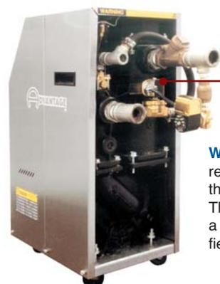
**WATER PURGE KITS...** removes process water from the process to the unit drain. The purge kit is supplied as a factory installed option or a field retrofitted kit.
