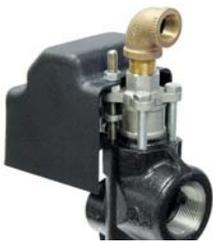
The Sentra® temperature control unit relies on an external source of cooling water. The patent pending **AVT™ (Advanced Valve Technology)** is the industry's first and only modulating cooling valve designed specifically for temperature control units. The **AVT™** cooling valve offers straight line temperature control by opening or closing in 2000 steps, from 0% to 100% to pass a precise flow to drain. This introduces cooling water from plant supplies with no water hammer
