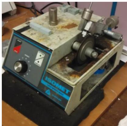
**Figura 2.1:** Sierra Buehler Isomet Low Speed Saw.
