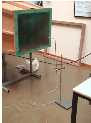
Figure 39: pitot tube and support
