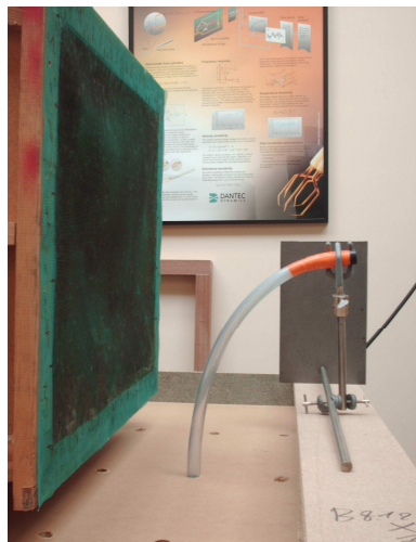
Figure 69: support and clamp, side view
