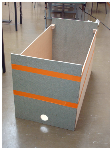
Figure 67: wooden box with sealed joints
