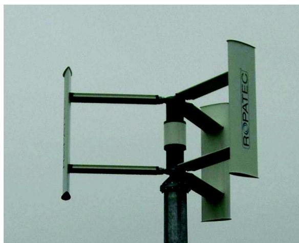
*Fig.16. Rotor Darrieus de palas rectas*
