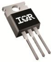
Figure 3.7: IRF60B217 with TO-220AB package
