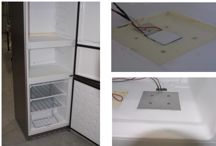
Figure 5. Pictures of the construction process of prototype 1.
