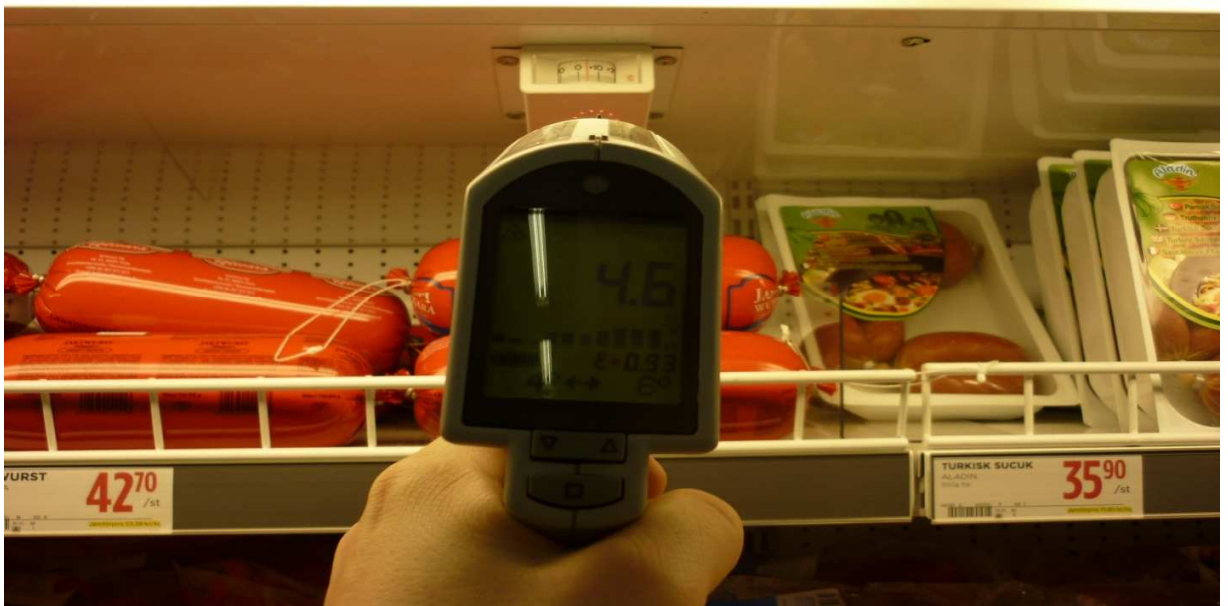
Figure 4; Laser gun measuring the temperature inside a refrigerated showcase
