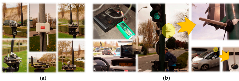
Figure 9. Different devices employed in order to implement the VANET WSN testbed: (a) infrastructure gateways and nodes; and (b) embarked transceivers.
