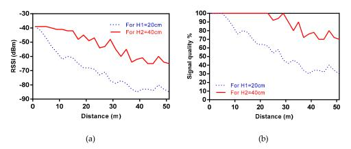
Figure 3. Difference at H<sub>1</sub> and H<sub>2</sub> between (a) RSSI values; (b) link quality.
