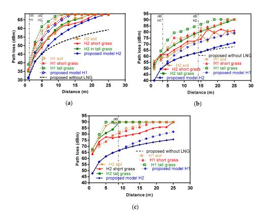
**Figure 2.** Path loss in agriculture fields at (a)  $F_1$ ; (b)  $F_2$ ; (c)  $F_3$ .
