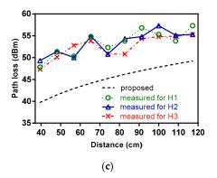
**Figure 1.** ComParison of the proposed model with path loss measurement results at frequency range (a) F<sub>1</sub>; (b) F<sub>2</sub>; (c) F<sub>3</sub>.
