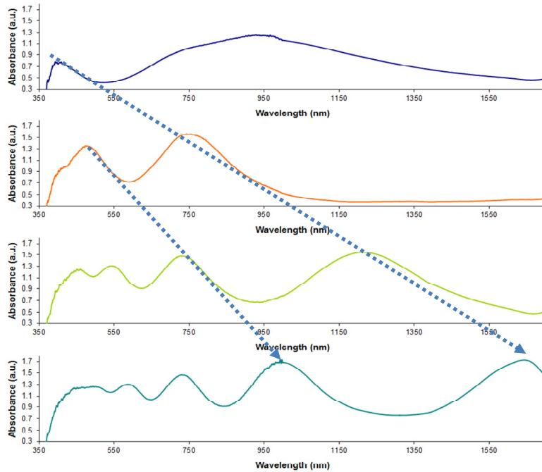
Fig. 3. Optical spectra of a LMR optical fiber device when the thickness of the supporting layer is increased. In this case, the supporting layer was a Layer-by-Layer assembled coating of [TiO<sub>2</sub>/PSS], and the number of bilayers from top to bottom was 10, 30, 50 and 70. Details about the fabrication process of these coatings can be found in [9]
