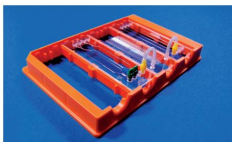
Fig. 72: Rhombic chamber chip in handling frame connected to PCR chip
