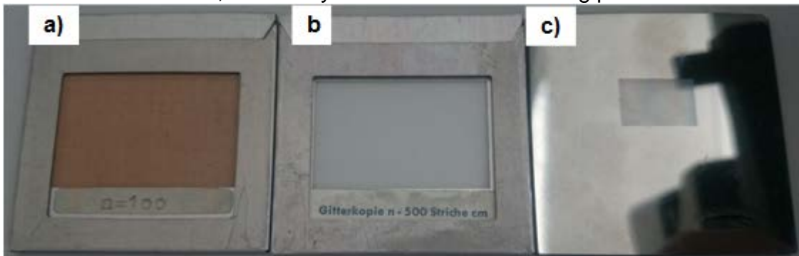
Figure 3.14- Calibration plates. From left to right: (a)100lines/cm, (b)500lines/cm and (c)1000lines/cm.
