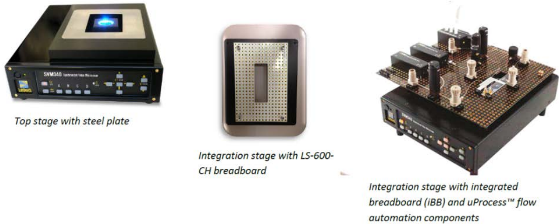
Figure 2.14- The three possible ways to integrate the imaging experiment with the SVM340 [14].
