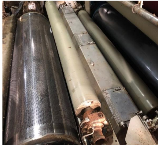
Fig. 33: Part of the press section of the PM4
