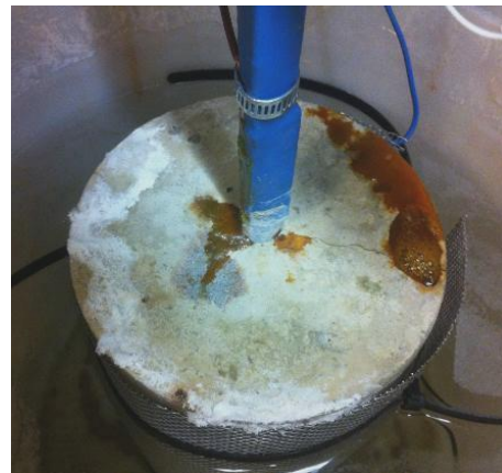
Fig. 8 Photo of corroding cylinder
