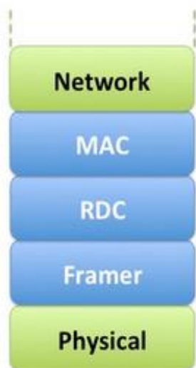
Figure 1.4: IEEE 802.15.4 protocol stack in ContikiOS (Extracted from http://anrg.usc.edu/contiki/index.php/MAC_protocols_in_ContikiOS )
