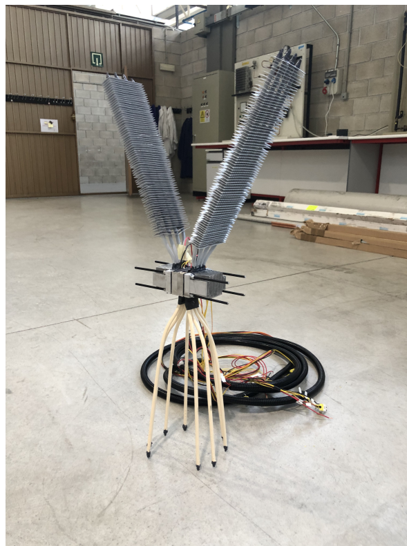
Figure 2. Designed thermoelectric generator composed of two thermoelectric modules and heat pipes as heat exchangers.
