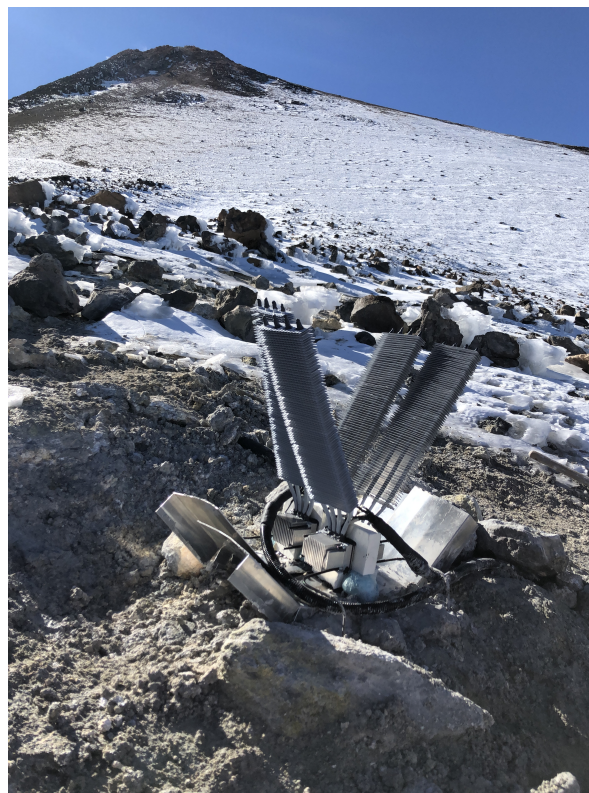
Figure 9. Prototype installed at Teide volcano on December 2019, composed of 4 thermoelectric modules.
