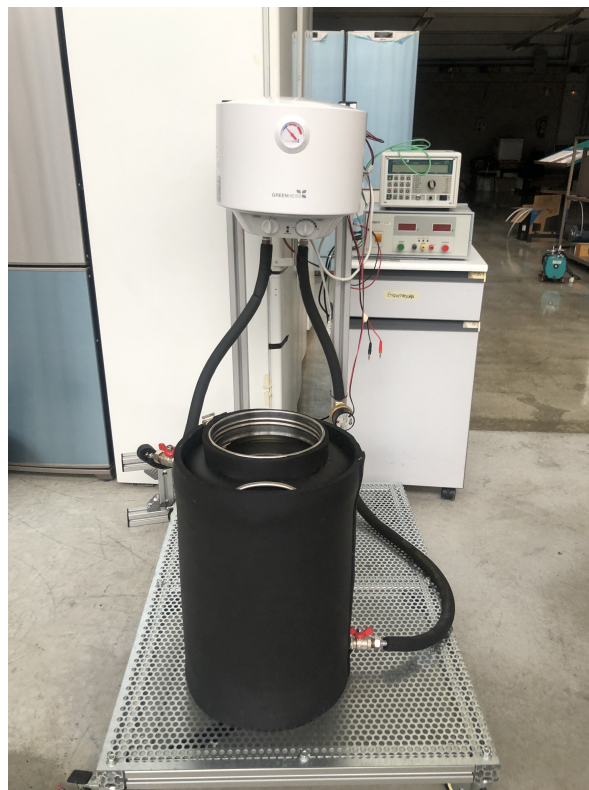
Figure 4. Thermal bath used as heat source in the laboratory experiments to determine the power generated by the designed prototype.
