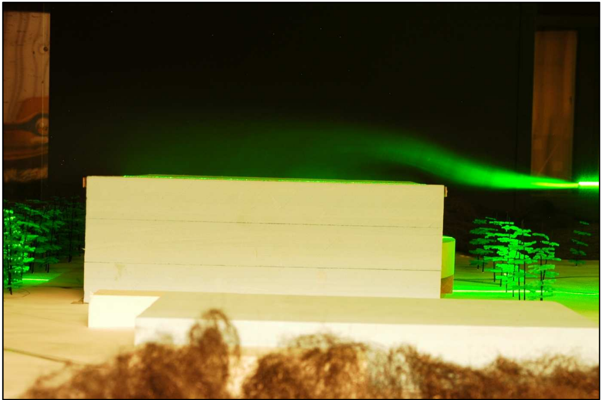
Figure 47. Photo of the smoke test with laser
