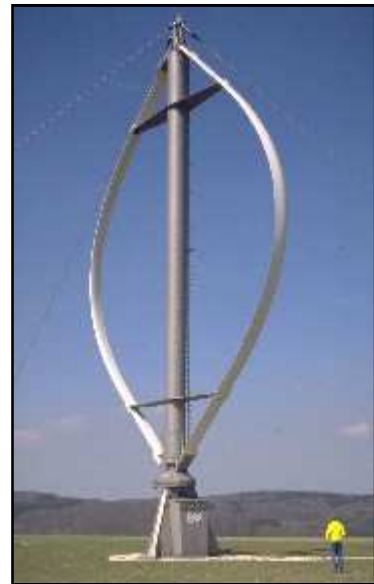
Figure 5. Darrieus wind turbine
