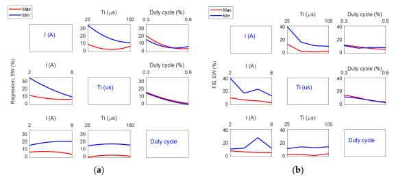
**Figure 12.** Interaction effects plot for EW in the case of positive polarity: (a) obtained from the regression [2]; (b) obtained with the proposed methodology using the FIS.
