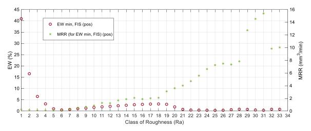
**Figure 18.** Values obtained from the technological table with the fuzzy inference system for the strategy of minimum electrode wear using positive polarity.
