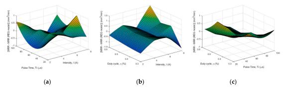
**Figure 8.** Difference between MRR (FIS model) and MRR (regression [2]) vs.: (a) Pulse Time and Intensity; (b) Duty cycle and Intensity; (c) Duty cycle and Pulse Time.
