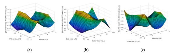
**Figure 7.** Difference between Ra (FIS model) and Ra (regression [2]) vs.: (a) Pulse Time and Intensity; (b) Duty cycle and Intensity; (c) Duty cycle and Pulse Time.
