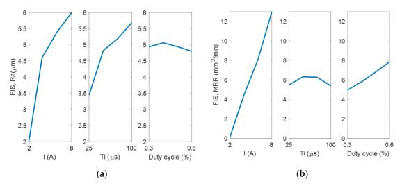
Figure 11. Main effects plot for (a) Ra and (b) MRR in the case of positive polarity, obtained using the FIS.
