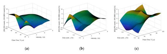
**Figure 6.** Difference between EW (FIS model) and EW (regression [2]) vs.: (a) Pulse Time and Intensity; (b) Duty cycle and Intensity; (c) Duty cycle and Pulse Time.
