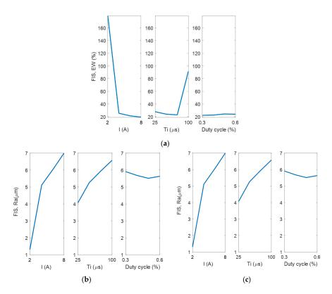
**Figure 14.** Main effects plot for **(a)** EW, **(b)** Ra, and **(c)** MRR in the case of negative polarity, obtained using the FIS.
