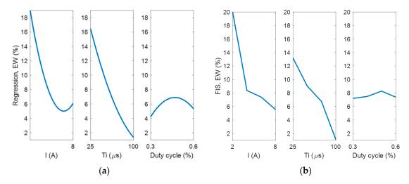
**Figure 10.** Main effects plot for EW in the case of positive polarity: (a) obtained from the regression [2]; (b) obtained by using the FIS.
