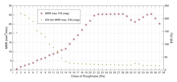
**Figure 17.** Values obtained from the technological table with the fuzzy inference system for the strategy of maximum removal rate using negative polarity.
