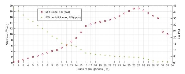
**Figure 16.** Values obtained from the technological table with the fuzzy inference system for the strategy of maximum removal rate using positive polarity.
