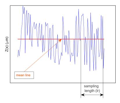
Figure 2. Roughness profile for determination of Ra parameter.
