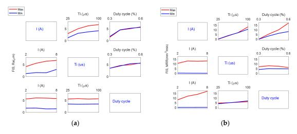
Figure 13. Interaction effects plot for (a) Ra and (b) MRR in the case of positive polarity, obtained using the FIS.
