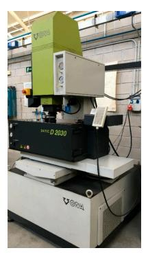
Figure 3. Electrical discharge machining (EDM) machine ONA Datic D-2030-S.
