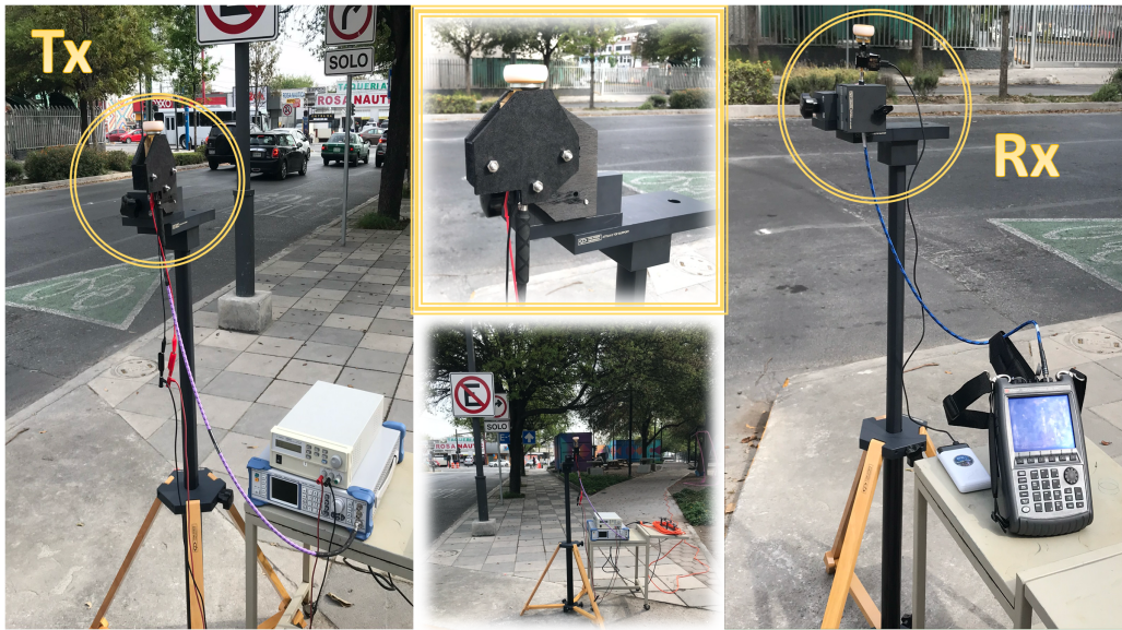
Figure 7. Collage of the measurement equipment used during the measurement campaign and detailed view of the transmitter system as well as the receiver composition.
