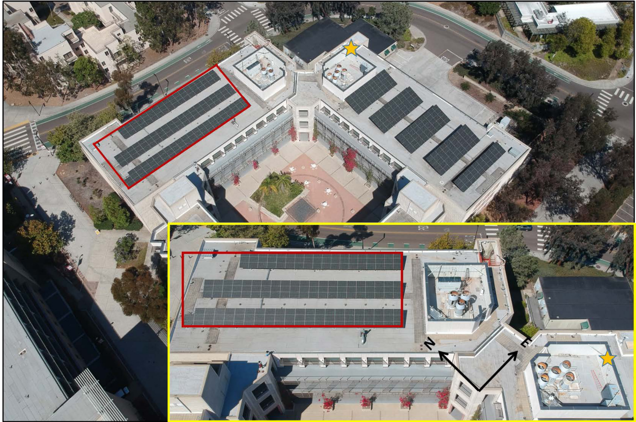
FIG. 2. Aerial view of the PV systems installed on EBU2 at UCSD. Plane view of the PV system (red rectangle) considered in the ramp estimate model is the inset at bottom right. The yellow star indicates the cloud speed sensor (see Sec. III C) located 30 m east of the lower right corner of the PV system. Copyright Drone Photo by Guang Chao Wang.
