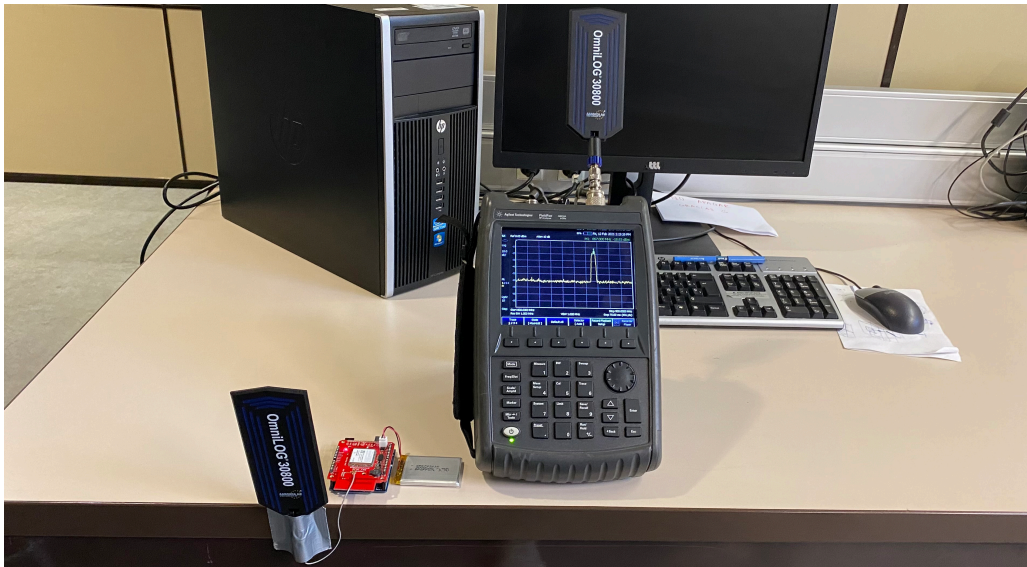
Figure 5.2: Spectrum analyzer and reader setup. [Own]
