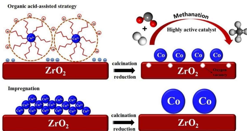
Figure 5. Proposed mechanism for the organic acid assisted methanation of CO 2 (Reproduced with permission from [76] ).
