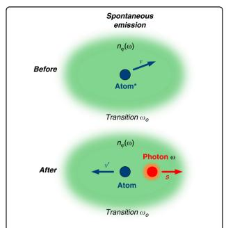
Fig. 1 Schematic of the spontaneous emission process inside NZI materials of refractive index  $n_{\varphi}(\omega)$  (green background). An atom (blue) moves around at a velocity v (v') before (after) spontaneous emission process. A photon (red) is being emitted after the excited atom relaxed in its ground state, in direction s
