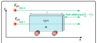
**Fig. 2 Schematic of Balazs gedanken experiment inspired by**<sup>48,49</sup>. The photon can either take path 1 inside the slab of mass M, length L and group index  $n_g(\omega)$  or follow path 2 in free space. The slab is supposed to move freely, without friction in the x direction
