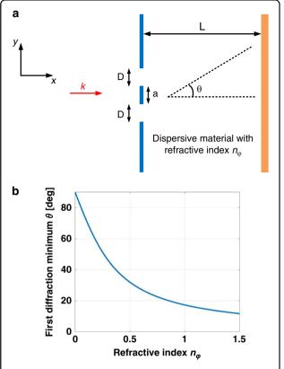
**Fig. 3 Young double-slit experiment within dispersive material. a** EM wave with k wavevector is sent on a double-slit with slit width D at a distance L from an observing screen. The distance between the slits is a. **b** First diffraction minimum as a function of refractive index. Wavelength is set to 500 nm for a separation width of a = 800 nm
