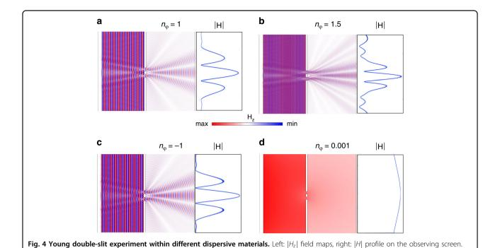
**a** Air ( $\varepsilon = \mu = 1, n_{\varphi} = 1$ ), **b** dielectric material such as glass ( $\varepsilon = 2.25, \mu = 1, n_{\varphi} = 1.5$ ), **c** a negative refractive index material ( $\varepsilon = -1, \mu = -1$ ,  $n_{\varphi} = -1$ ) and **d** an ENZ material ( $\varepsilon = 1 \times 10^{-6}, \mu = 1$  and n = 0.001). Wavelength is set to 500 nm for a separation width of 800 nm
