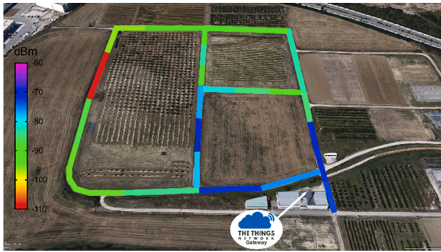
Fig. 30. LoRaWAN 868 MHz coverage map for tractor to gateway communication.
