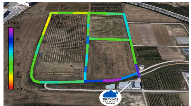
Fig. 19. LoRaWAN 868 MHz coverage map for farmer to gateway communication.
