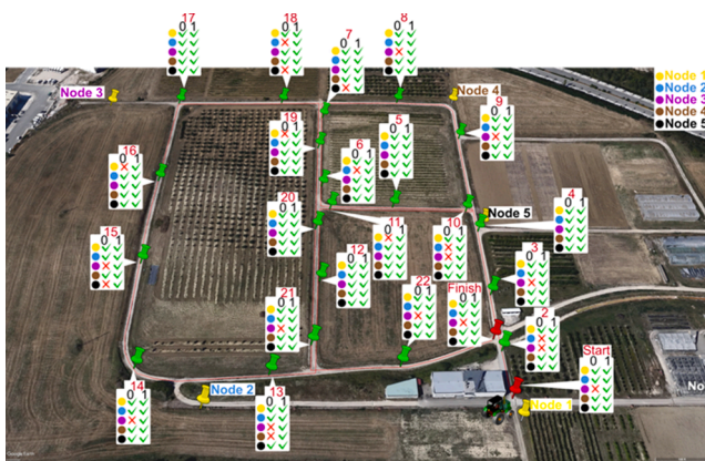
Fig. 24. LoRa 868 MHz received packets by the tractor at different locations.
