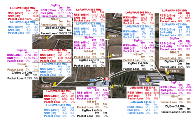
Fig. 8. Average RSSI, SNR and packet loss using different wireless technologies at different locations and heights.
