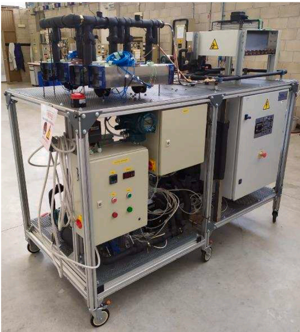
Fig. 2. Experimental vapour compression refrigeration plant.
