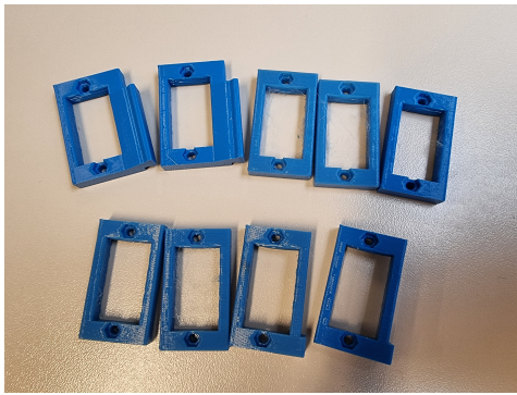
(a) Different tests to get the adequate hole size
