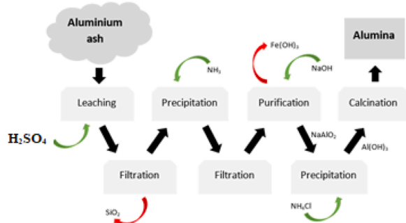
Fig. 6. Summary of the process carried out by Benkhelif et al. (2022) for the extraction of alumina from a waste slag.
