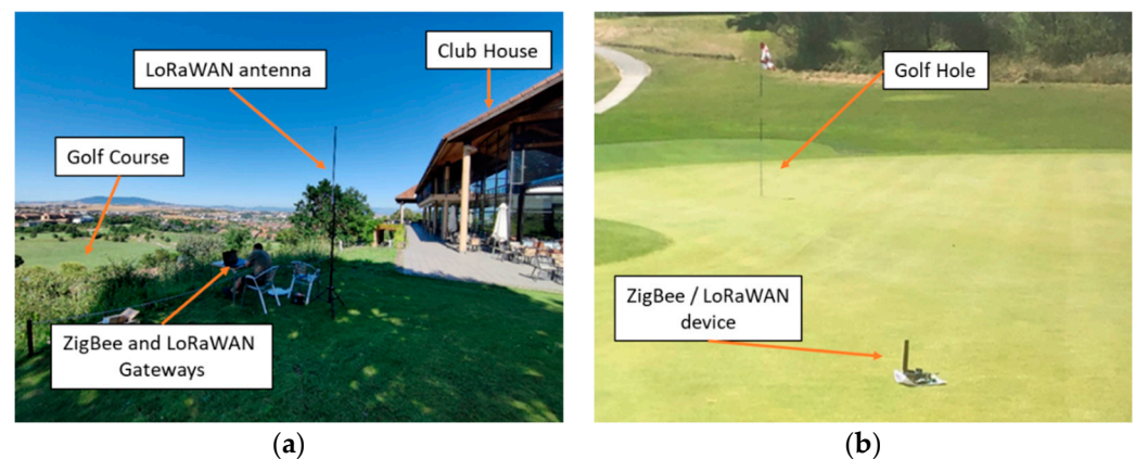
Figure 12. (a) Gateways deployment in front of the Club House; (b) Node deployment on the Green.
