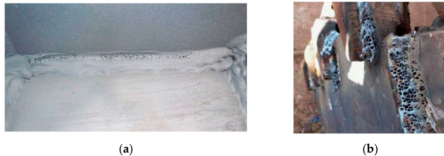
Figure 4. Porosity: (a) surface porosity uniformly distributed along the weld seam is produced because the displacement angle is too large (excessive slope); (b) porosity occurred because the gun is too far away from the workpiece or the voltage has been insufficient at the welding distance.
