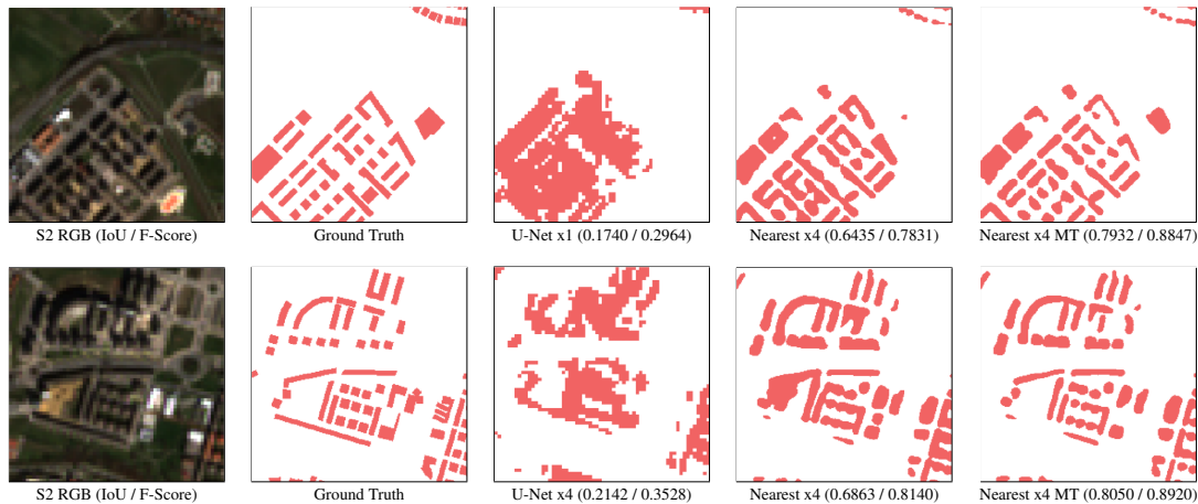
Fig. 2. Visual comparison between the original U-Net architecture trained using only the first trimester, and the proposed modification with nearest-neighbor input up-scaling trained using both single multi-temporal data.
