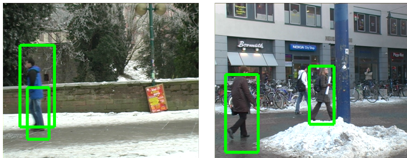
Figure 1: LEFT: Image where the algorithm detects two objects where there is only one (using Gall). RIGHT: Image with one missing object(Wenzel).
