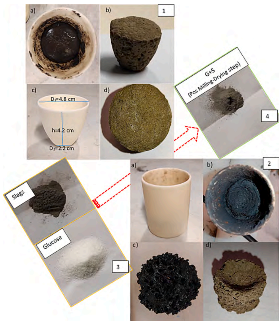
Fig. 1. Ceramic foam prototypes made with two molds using the experimental process. 1-a) G/S paste (0.7 wt%) melted and homogenized inside a truncated conical ceramic mold for high temperatures 1-c). 2-a) cylindrical ceramic mold, 2-b)-c) green carbonaceous foam, 2-d) cylindrical prototype of the ceramic support filter at 1200 \text{ }^\circ\text{C} . (For interpretation of the references to colour in this figure legend, the reader is referred to the web version of this article.)
