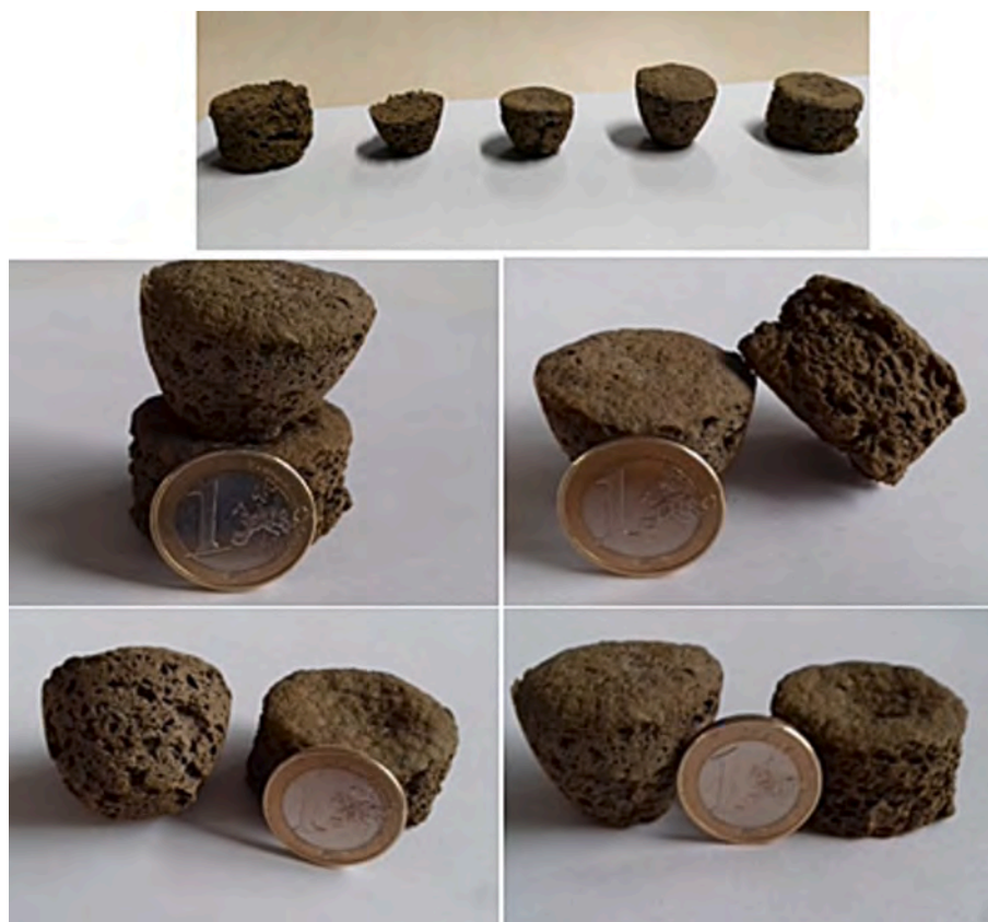
Fig. 2. Prototypes of ceramic foam filter supports synthesized from aluminum saline slags with several composite morphologies.
