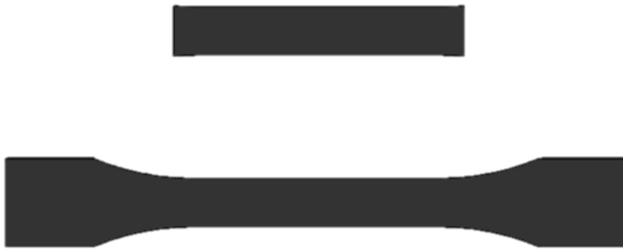
Figure 22. ISO 527-2 comparison with the narrow center subjected to TO
