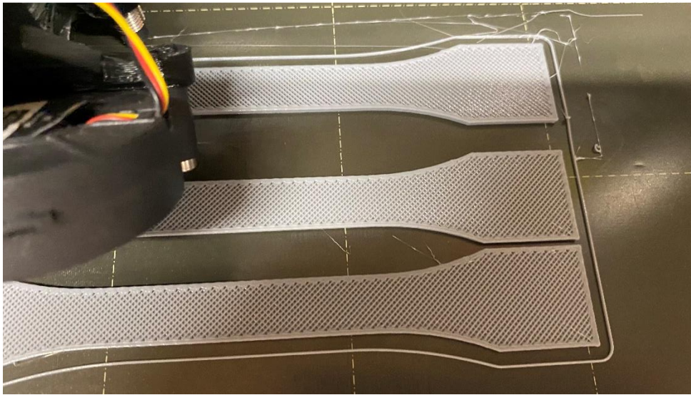
Figure 25. Detail of infill density when printing
