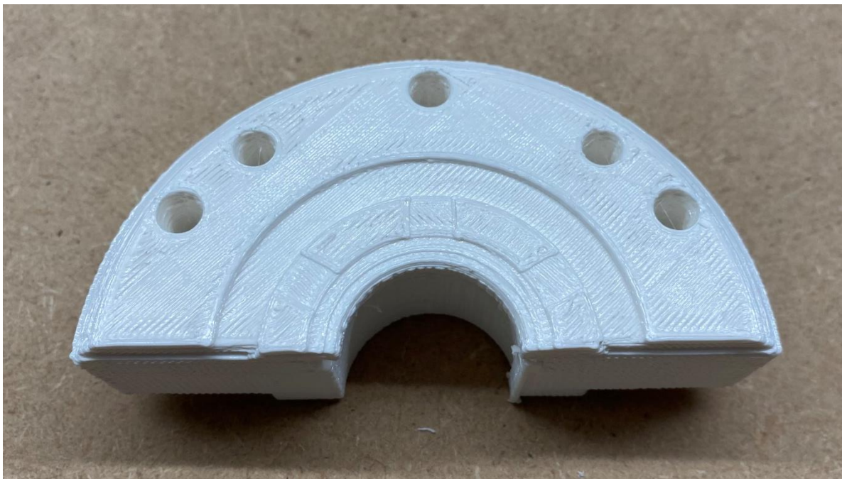
Figure 87. Mold component 3D printed with PLA
