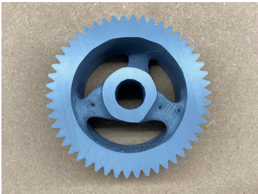
Figure 68. Entire gear 1000N topology study result 3D printed front view
