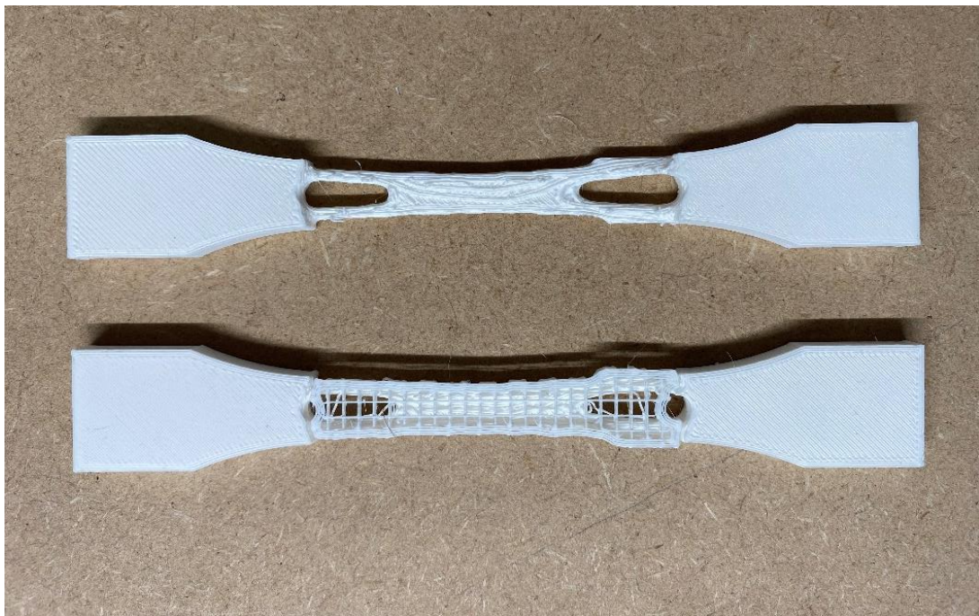
Figure 34. Support generated by Cura
