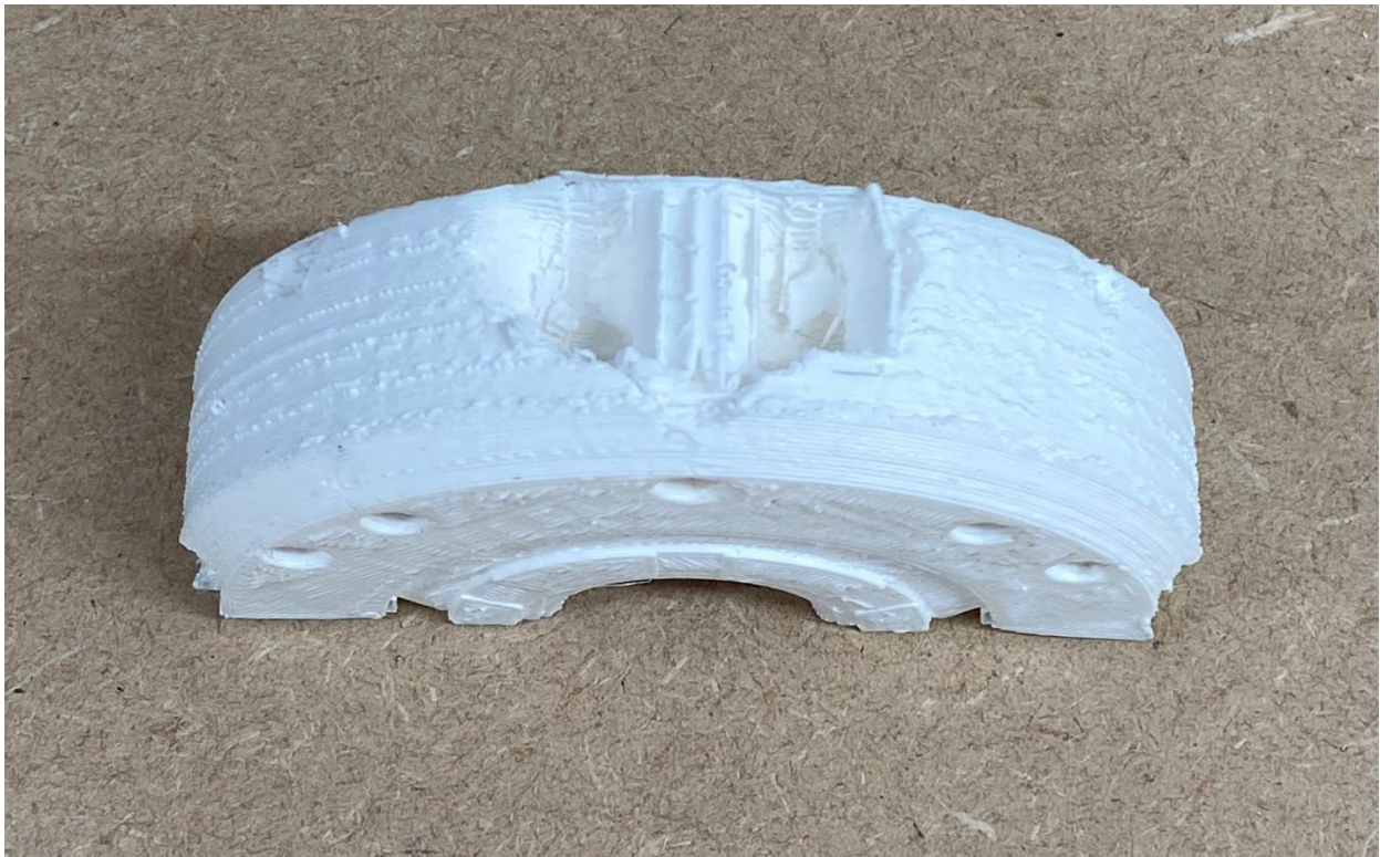
Figure 86. Mold component topologically optimized design 3D printed with PLA
