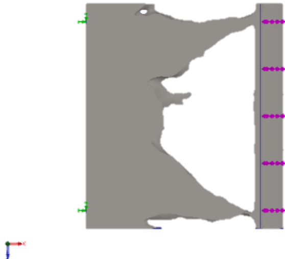
Figure 67. One tooth of gear 1000N topology study result front view
