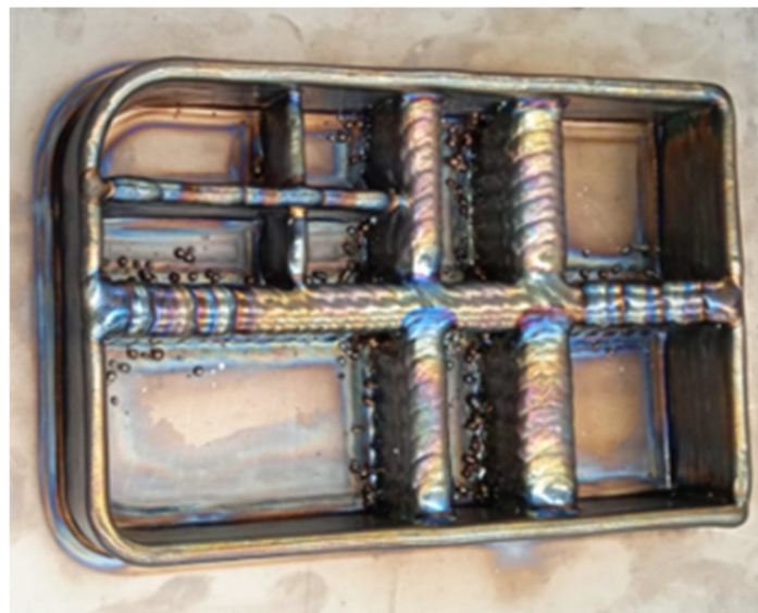
Figure 6. Photograph of the real titanium demonstrator in preform format after arc-DED printing.
