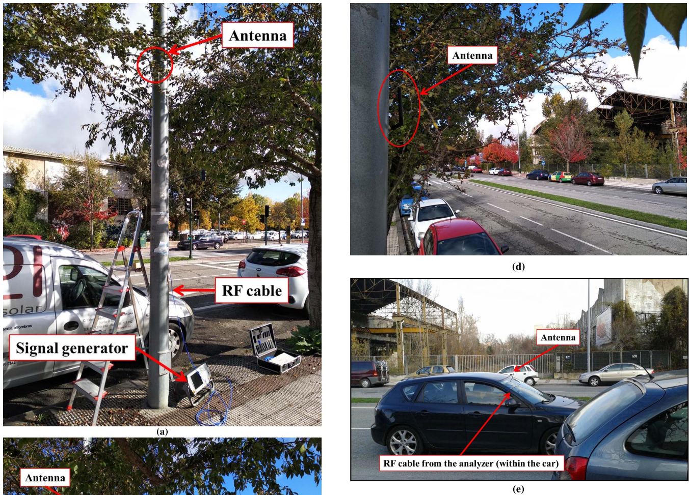
Fig. 15. Real pictures of the equipment deployment: (a) Deployment on a lamppost; (b) Left hand view of the scenario under analysis; (c) Right hand view of the scenario under analysis; (d) Detail of the deployed antenna; (e) Deployment on a conventional car.
