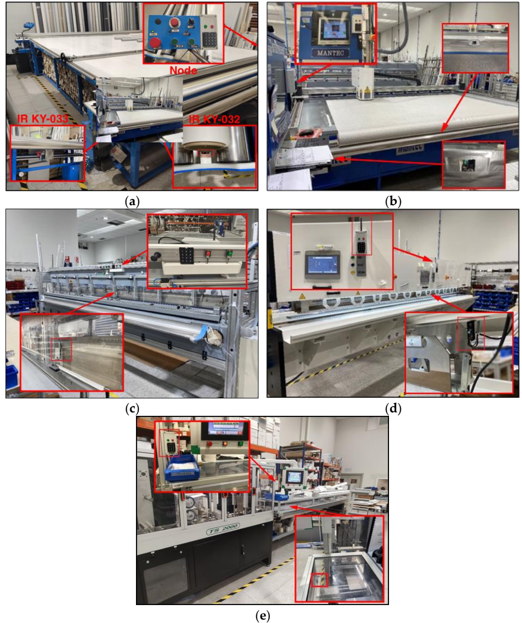
Figure 13. The implemented nodes at different workstations: (a) knife cutting machine; (b) laser cutting machine; (c) thermal welding machine 1; (d) thermal welding machine 2; (e) automatic slat machine.
