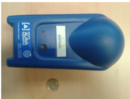
FIGURE 4. EME Spy 121 personal dosimeter used for the campaign of measurements within the buses
