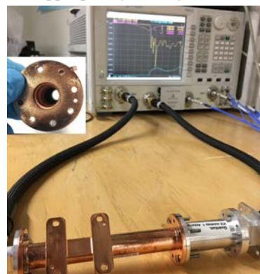
Fig. 7. 3D printed SatCom circular waveguide filter measurement.
