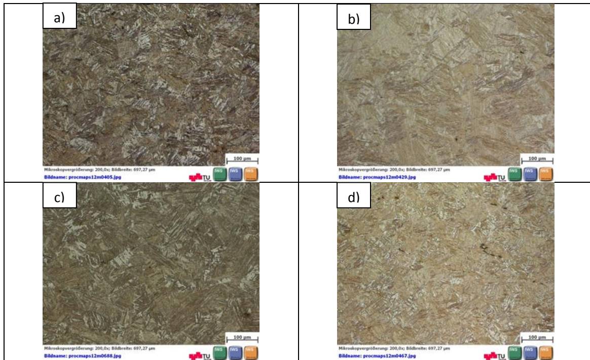
Fig.34. Light optical micrographs showing the microstructure of the material after compression test at 1050°C in the middle (a) strain rate of 0.01s^{-1} , (b) strain rate of 1s^{-1} , and in the edge (c) strain rate of 0.01s^{-1} , (d) strain rate of 1s^{-1} . Magnification 200x.
