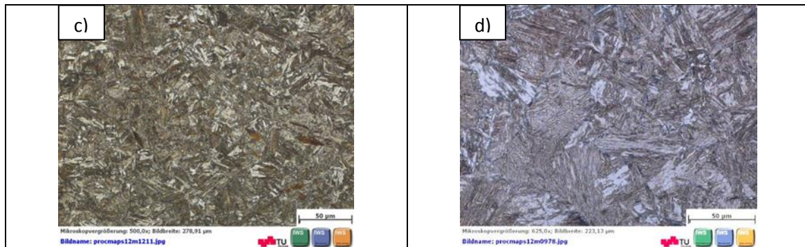
Fig.25. Light optical micrographs showing the microstructure of the material after compression test at 950°C in the edge (a) strain rate of 0.01s^{-1} , (b) strain rate of 1s^{-1} , (c) strain rate of 10s^{-1} , (d) strain rate of 80s^{-1} . Magnification 500x
