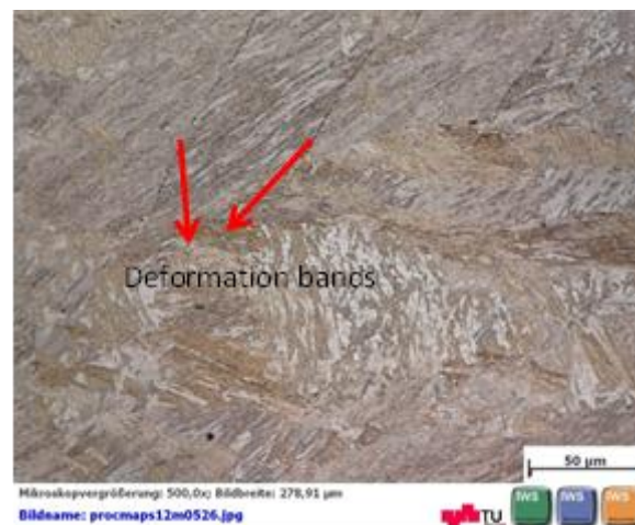
Fig.41. Deformation bands in a compression test carried out at 750°C. This picture was taken in the edge of the sample.
