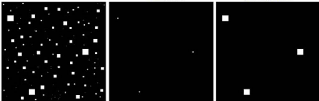
Figure 1.1 (a) Image of squares of size 1, 3,5,7,9, and 15 pixels on the side. (b) Erosion of (a) with a square structuring element of 1's, 13 pixels on the side. (c) Dilation of (b) with the same structuring element.
