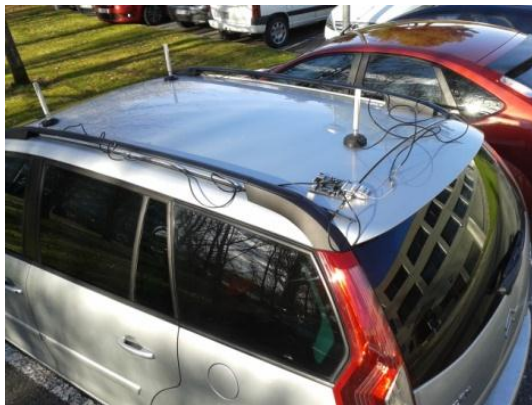
Figure 14. View of the set up for the experiments, with the antennas magnetically mounted on the car roof.
