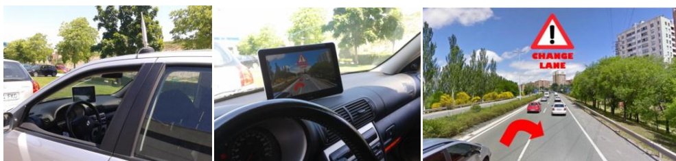
Figure 9. Location of external antenna (left image) and tablet (middle image), and example action suggestion (right image).
