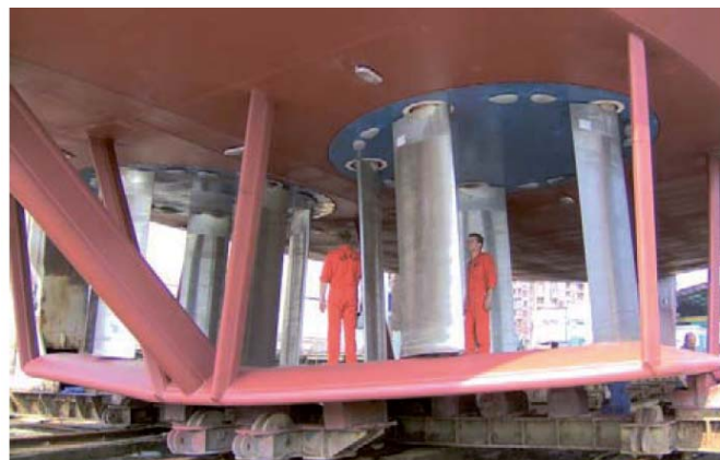
Figure 4.5: Voith Schneider propulsion concept with vertical axis technology
