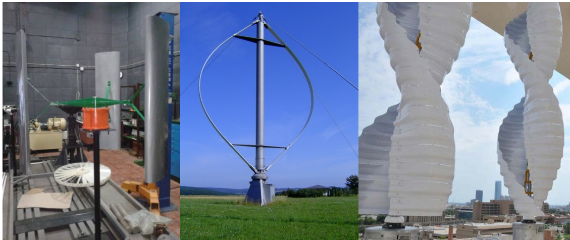
Figure 4.3: Straight-bladed Darrieus rotor on the left, Darrieus rotor in the middle and Savonius wind turbine on the right
