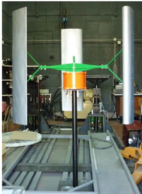
Figure 9.1 Vertical axis wind turbine prototype in the laboratory
