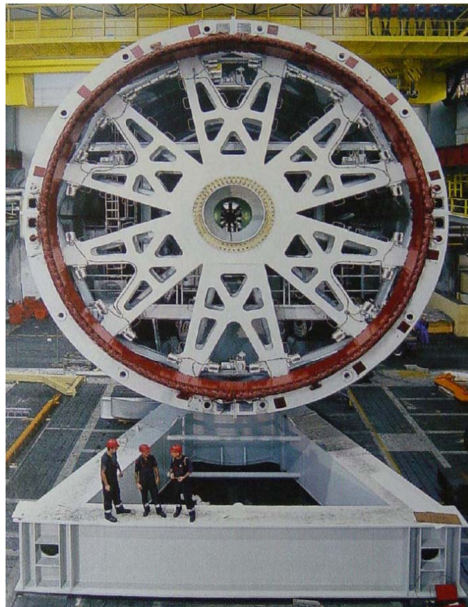
Figure 6.3.2: Generator of a direct drive PMSG of a 5MW wind turbine[4]
